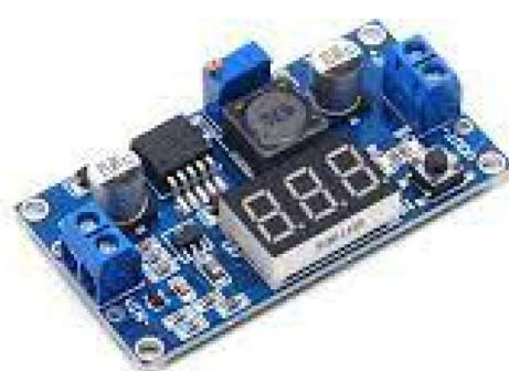
Slika 14 : Step-down converter
